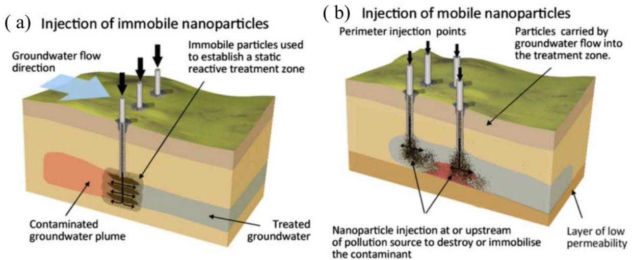
**Fig. 4** Schematic representation of nanoparticle application showing how (A) immobile nanoparticles and (B) mobile nanoparticles are injected into the subsurface for groundwater treatment (modified from Crane and Scott 2012) (Grieger et al. 2015)
