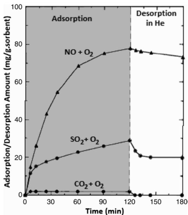
**Fig. 3** Adsorption/desorption profile of CO<sub>2</sub>, NO<sub>x</sub> and SO<sub>2</sub> on carbon nanotubes at 25°C (Long and Yang 2001)
