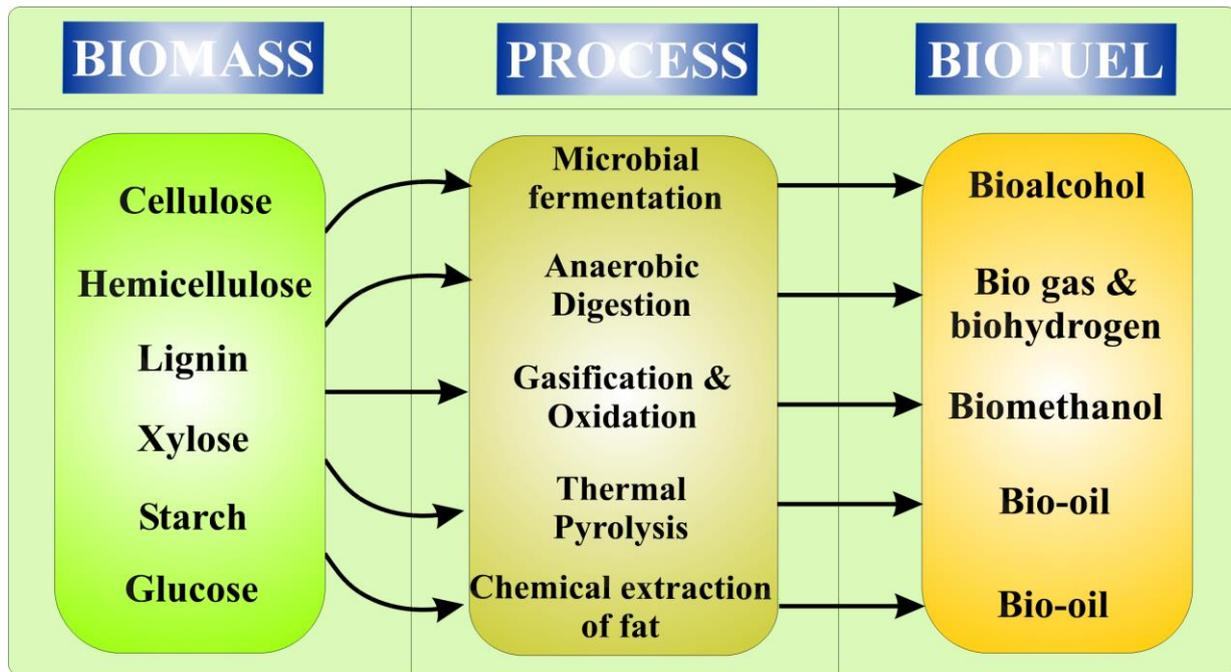
**Fig. 2** Schematic diagram depicting some common production processes of second and third generations’ biofuel from biomass feedstock of aquatic weeds.
